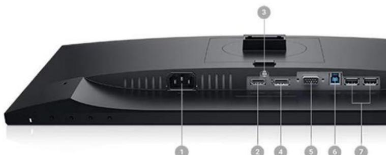
**Ports & Slots:** 1. Power Connector | 2. HDMI Port | 3. Stand Lock Feature | 4. DisplayPort | 5. VGA Connector | 6. USB Upstream Port | 7. USB Downstream Ports
